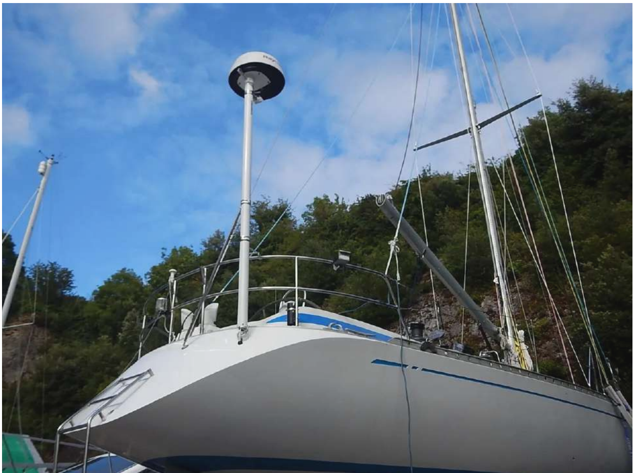
I decided upon the longer 2.5 Meter pole length for our installation. Scanstrut also offer a shorter pole for smaller boats or different mounting solutions ondeck rather than mounting onto the
