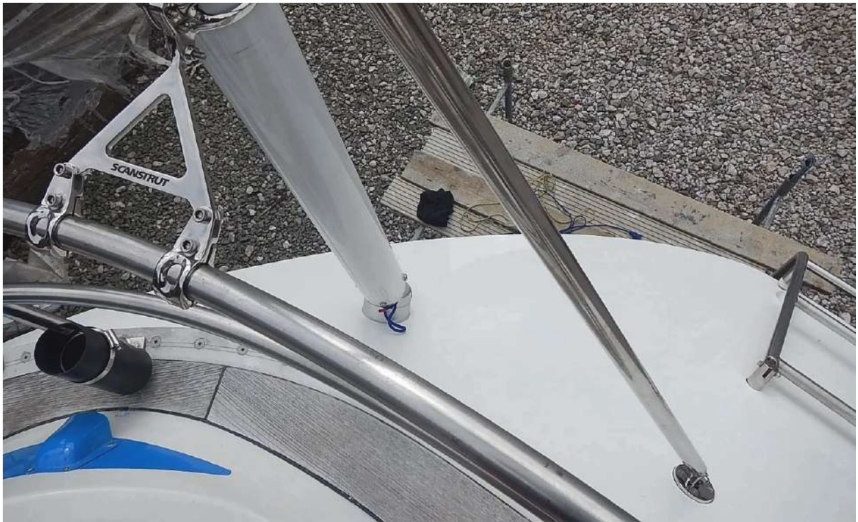
The view from above the pushpit looking down at the transom face. Showing the base of the Scanstrut pole mounting and side brace support.
